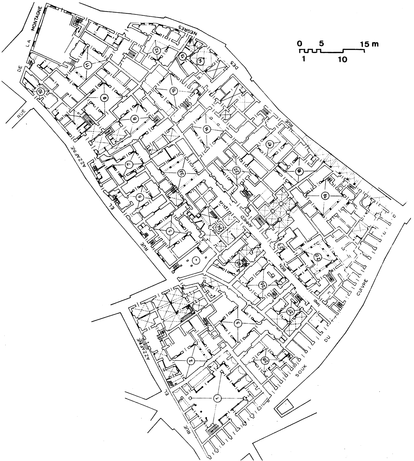
Figure 5. Tunis Plan of block no. 200 showing buildings abutting each other. Source: Association Sauvegarde de la Medina, Tunis, 1968.
